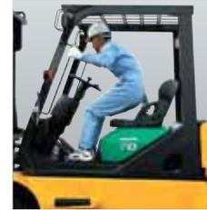
KOPS Plus is activated when the operator leaves the seat for more than three seconds.
