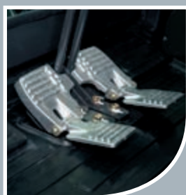
The new, ergonomic, cast aluminium travel pedals ensure smooth, confident travel control of the machine.
