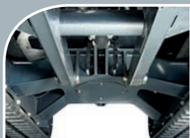
The new X-frame undercarriage offers better ground clearance and easy shedding of debris.
